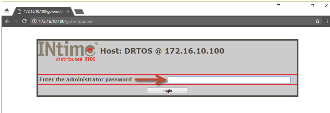
Figure 2.4 - Password screen of the target platform's built-in web-server.
