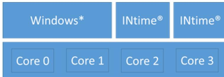
*Figure 1: Explicit hardware partitioning of OS environments with Microsoft Windows and INtime on a 4-core processor.*
