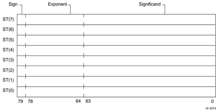
**Figure 6-9. Numeric Coprocessor Stack of Numeric Data Registers**
