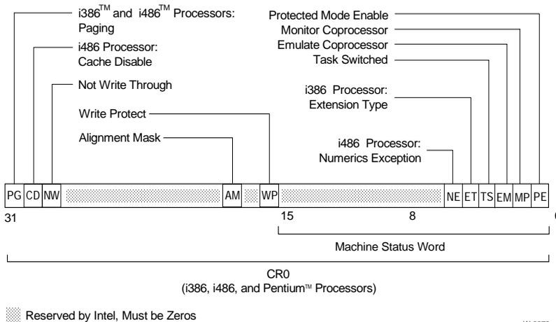
**Figure 6-8. Control Register 0 of Intel386, Intel486, and Pentium Processors**
