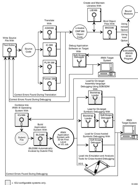
Figure 1-1. 32-bit Protected Mode iRMX Application Development
