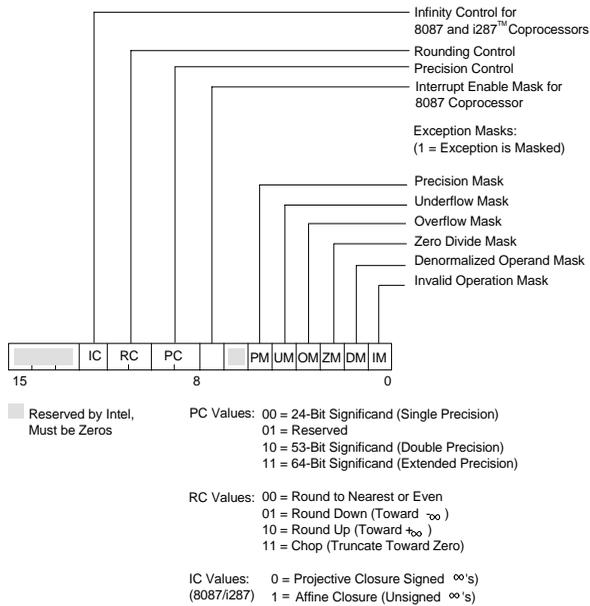
**Figure 6-12. Numeric Coprocessor Control Word**
