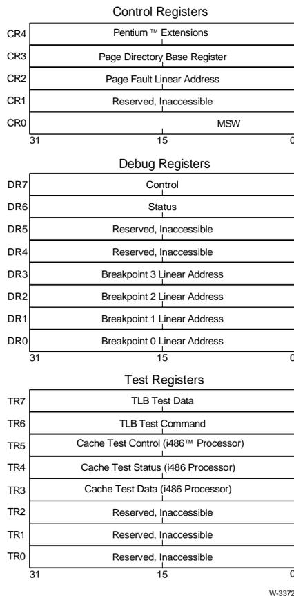
**Figure 6-7. Control, Test, and Debug Registers of Intel386, Intel486, and Pentium Processors**
