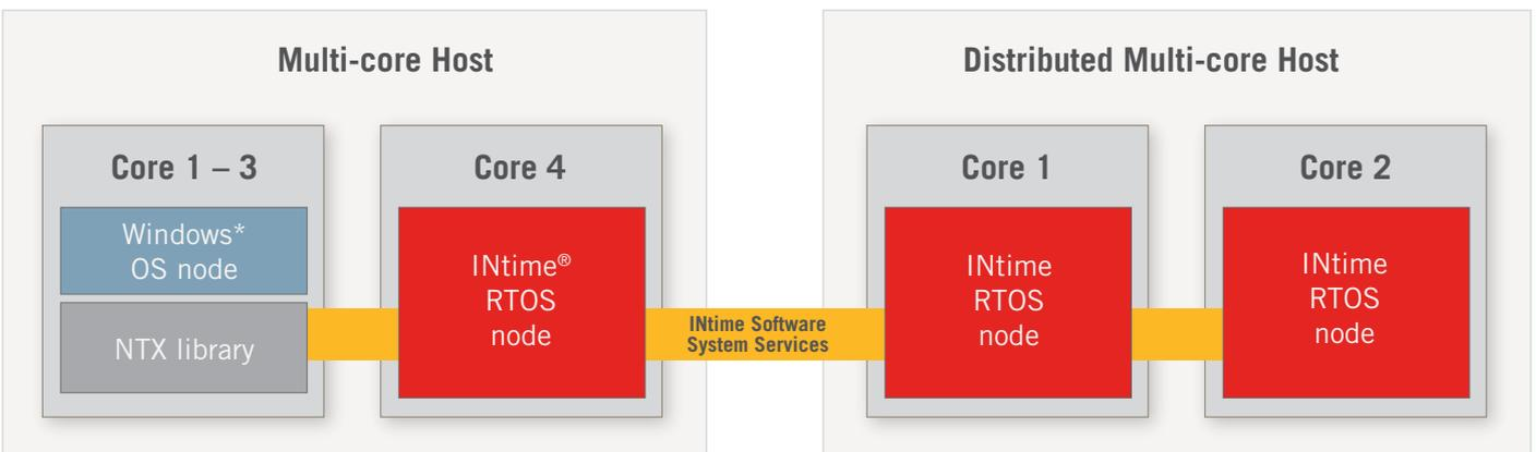
Figure 1. Independent OS instances with distributed system services.
