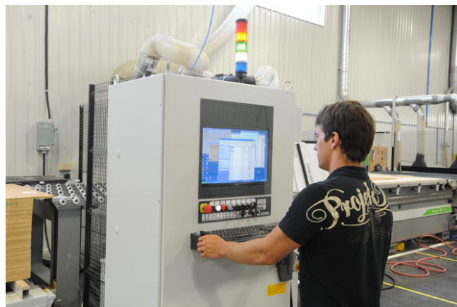
Figure 2. The Biesse Group's Rover Gantry machine's HMI runs on Microsoft Windows.
