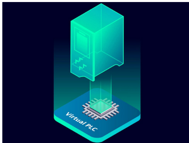
Figure 2. Virtual PLCs (vPLCs) like the Siemens SIMATIC S7-1500 can be implemented as workloads on partitioned multicore processors, paving the way for industrial PCs to operate as multi-function automation controllers. (Source: Siemens Blog )
